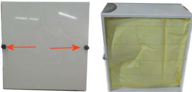
2. Slide the filter bag off the inlet collar and remove. The HEPA filter is housed behind a protective grill secured with 2 thumb wheel nuts.
