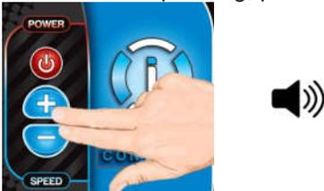
Hold for 10+ seconds; when panel is beeping continuously, release buttons .
